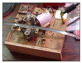
First off was David Demonstrating a band-saw blade sharpening device. He had constructed it using scrap from his copious store of 'It might come in useful' items. The whole set up looked distinctly Heat Robinson, but by gum it worked like a wizard! The contraption functioned automatically and could sharpen a band-saw blade in less than three minutes saving both money and Earth resources. Sorry Amazon.
